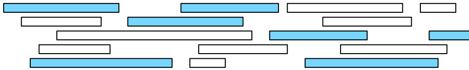
A set of intervals. The seven shaded intervals form a tiling path.
